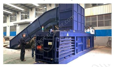
The semi-automatic plastic baler/paper baler is widely used to compress almost all the loose materials like paper, cardboard, OCC, ONP, books, magazines, plastic bottles, plastic film, textile waste, alfalfa, hays, cans, tins and aluminum scraps etc.
