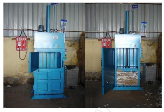
The waste paper baler is divided into single cylinder and double cylinder. Its main structure is the same. The difference is that the number of hydraulic cylinders of the two balers is different.
