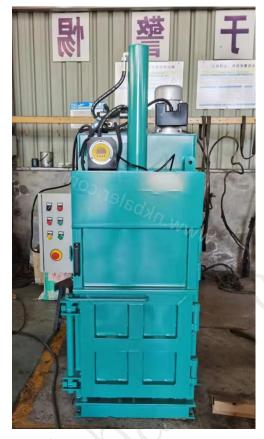
NK6040T10 Waste Paper Balers is wide used to compress loose materials like waste paper (cardboard, newspaper, OCC etc), plastic waste like PET bottle, plastic film, crate, it can also be used for straw;
