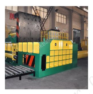
Y81 Scrap Metal hydraulic metal balers are applicable in steel plants, recycling companies, ferrous& non-ferrous smelting industry to press metal scraps (steel, copper, aluminum, stainless steel, discarded automobiles).
